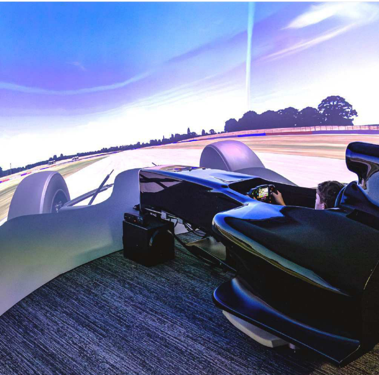
Focus simulators utilise real chassis and six-metre, 180 degree screens for the ultimate immersion experience
